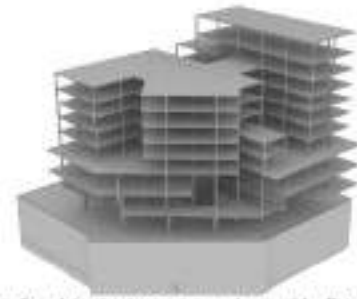
5. Complete simple 7.2x7.2m column grid + flat slab
